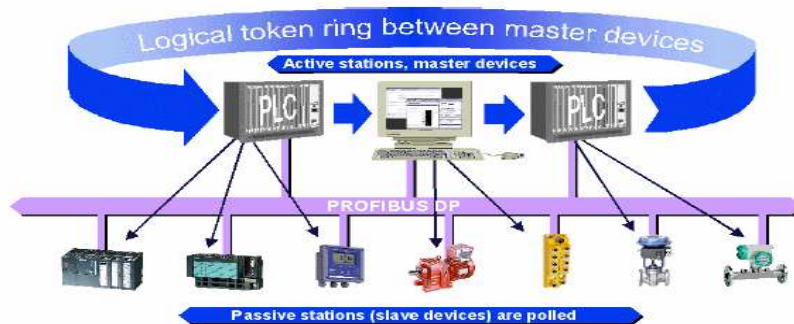
Fig. 5: PROFIBUS configuration with active masters and slaves
